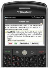
QSI's TEAMATE application translates results from diagnostics, automatic tests, and tests conducted by the technician into clear instructions on the action to be taken next.
