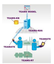
TEAMS-RDS used for remote troubleshooting and TEAMATE on a standalone portable computer used for onsite maintenance. Information on the standalone computer can be periodically synchronized with the server.
