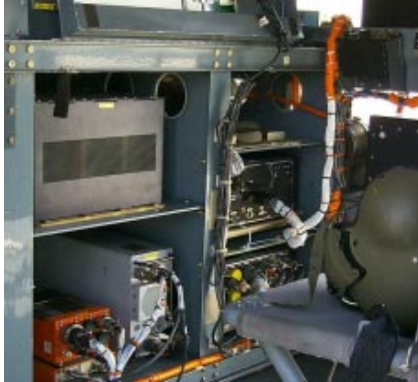
Figure 9 - TEAMS-RT computer installed on RASCAL.
