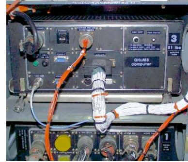
Sikorsky UH-60 on-board computer hosting TEAMS-RT. The QSI software uses the TEAMS model to perform continuous real-time diagnostics.
