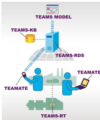
TEAMS-RDS used for remote troubleshooting and TEAMATE on a standalone portable computer used for onsite maintenance. Information on the standalone computer can be periodically synchronized with the server.
