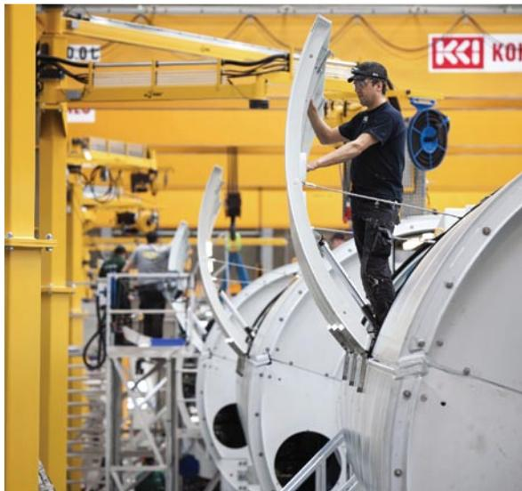
**Fig. 3: A Siemens worker during the inspection of the wind turbine nacelle in the production facility in Brande, Denmark.**
