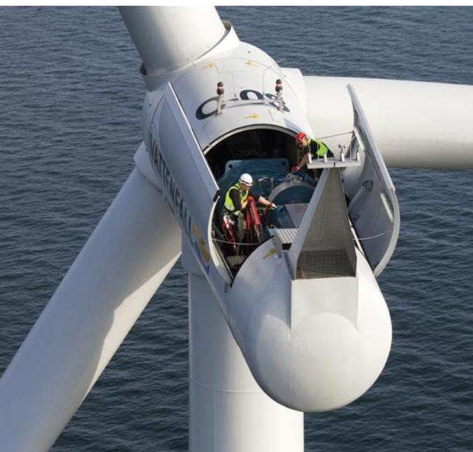
Fig. 7: Close-up of the rotor hub and opened gondola of a wind turbine at the Swedish offshore wind farm Lillgrund, type SWT-2.3-93 with a rating of 2.3 megawatts (MW).
